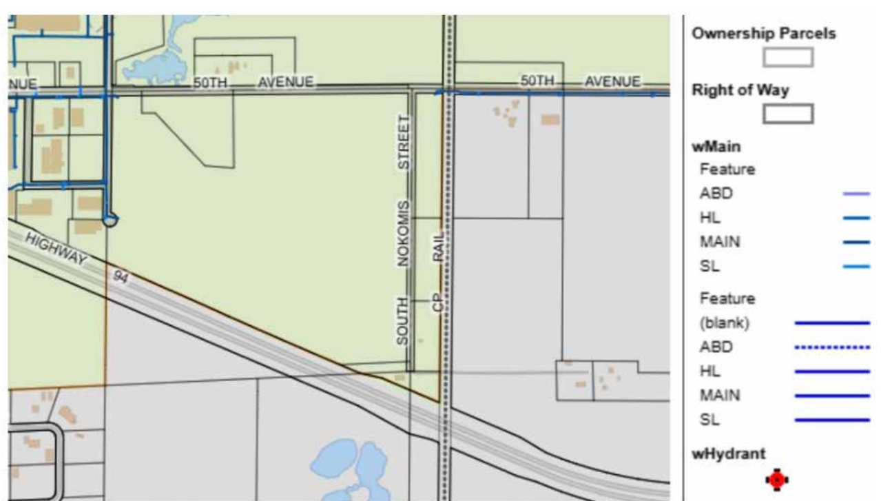
Alexandria Light & Power municipal water infrastructure near the site. Main size, pressure, and extension requirements require provider confirmation.
